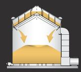
Step 3. When grain has dried to a predetermined temperature, the dump chutes open automatically, letting 1/4 of the dried grain in a 36', or 1/3 in the 24' or 30', fall into the cooling and storage area. The drying chamber is then automatically refilled, and drying continues until the grain supply is empty.
