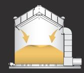
**Step 3.** When the column of grain has dried to a predetermined temperature, the fan(s) and heater(s) stop, and the operator manually opens the dump chutes letting the hot dried grain fall into the cooling and storage area below. The drying chamber is then manually refilled, and the operator can start the next batch drying.
