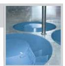
Self cleaning divider hopper separates the heating and cooling sections while preventing build-up of particulate matter.
