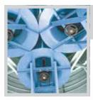
Internal inline, mixed flow centrifugal blowers deliver high volumetric airflow to the pressure heat and vacuum cool sections. **SEE PAGE 10 FOR MORE INFO.**
