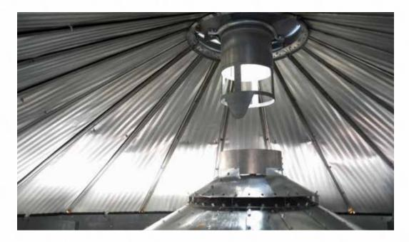
Grain moves down out of the garner area, and enters 12-3/4 inch wide grain drying columns in the heat section of the dryer.
