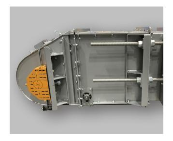
Tail section features spiral wing pulleys with plow and flipper reloading mechanism to automatically reclaim spilled material.
