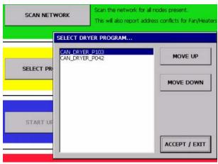
9. Press the START UPLOAD button and wait until all the boards are updated. In the future you do not have to press START UPLOAD on the upload status screen anymore. That redundant button has now been removed.
